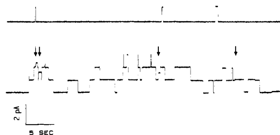
FIGURE 2: Single-channel activity induced by gramicidin A in DPhPC/decane membranes before and after addition of 8 \mu M Triton X-100 (Calbiochem). (Top) Control, before Triton addition. (Bottom) Results obtained after Triton addition (this trace was recorded \sim 3 min after the top trace). Channel currents are upward. In both traces, note the uniform amplitude of most channels. Some mini channels are denoted by arrows. Addition of Triton X-100 leads to an increased channel appearance rate and channel duration as well as a decreased amplitude of the single-channel current steps and an increased mini channel frequency. Filtered at 100 Hz.
